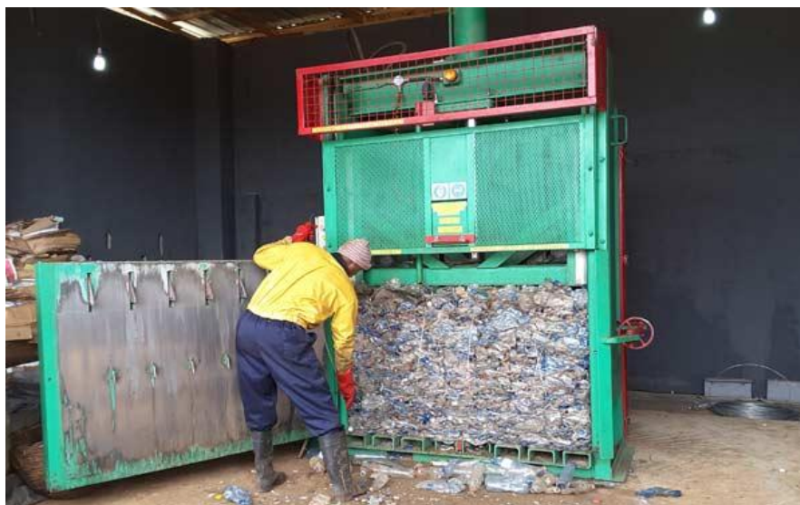
Figure 6. Collected PET plastic bottles undergoing machine compression [9]
